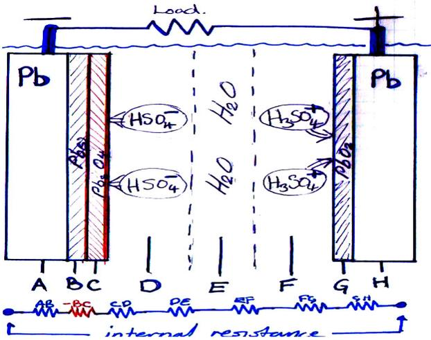
The red resistor in the series indicates where the dipole may exist.
